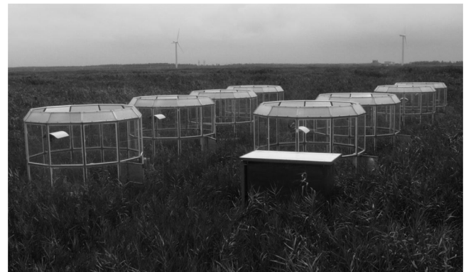
Fig. 3. Appearance of the open-top chambers (OTCs) applied in the simulated warming experiment conducted in the reclaimed salt marsh.
